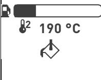
190 °C   | <b>Purging process is carried out</b><br>Adhesive nozzles are open, pressure has built in the adhesive cartridges. Display of the current status.                                                                                                                                                                                                                                       |
