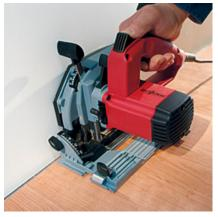
Perfect edging: the circular saw's spacers enable you easily to make exact expansion joint cuts with widths from 13 mm (1/2 in.).
