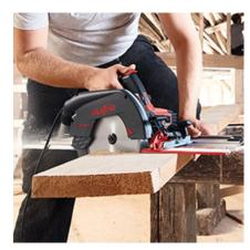
One-stop solution: with the crosscutting system, the machine is permanently attached to the guide track.
