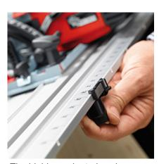
The highly graduated scale permits very precise angle setting.
