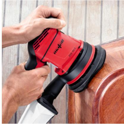
The compensating soft interface pad enables you to produce an outstanding finish on concave and convex surfaces. The foamed material smooths out any unevenness and ensures consistent sanding outcomes.
