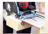
An ideal application for guide L is cutting structural timber to length, with a max. cutting depth of 82 mm and a max. cross-cutting length of 370 mm.
