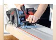
Ripping with a guide rail or parallel fence and an ample cutting depth. The two high-performance 18 V batteries of the K 85-18 combine to deliver a sustained output of 36 V.
