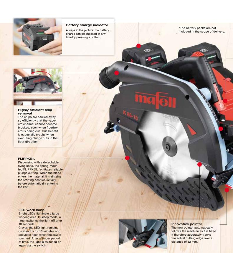
The K 85 / K 85-18 saws are perfectly equipped to meet the future challenges of the woodworking trades. Not only in view of their exemplary material and build qualities, but also thanks to their well-conceived user-friendliness and compatible dual-battery technology.
