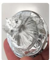
The image to the left is a fully consumed foil – there is some product in the centre, but the outside 'ring' has no residue on it. Give the applicator gun a good final squeeze, when fully dispensed, and there will be little adhesive/sealant remaining.
