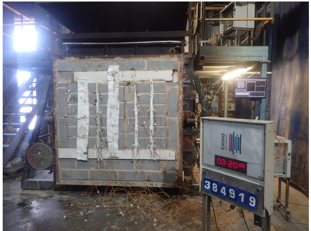
The unexposed face of the wall construction after a test duration of 200 minutes
