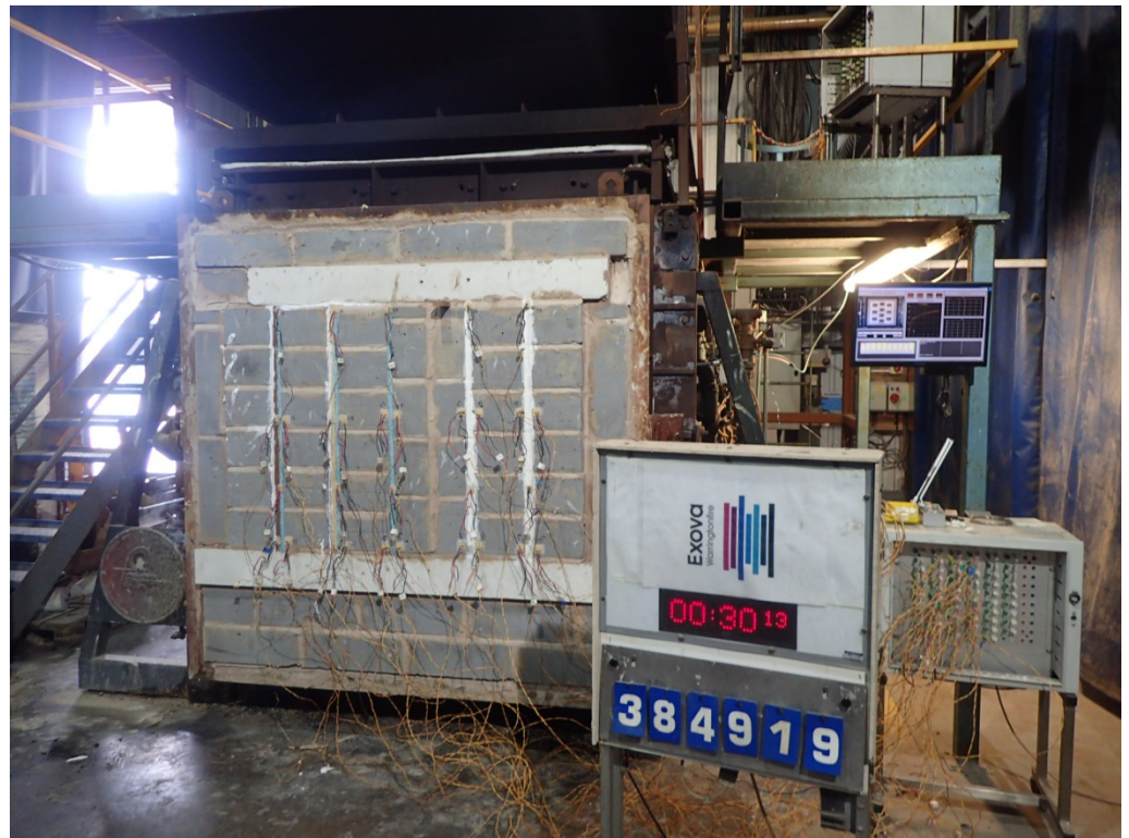
The unexposed face of the wall construction after a test duration of 30 minutes
