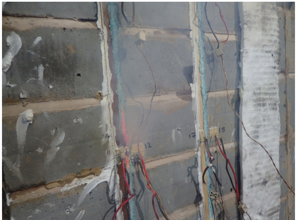
Integrity failure seen from Specimen A after a test duration of 179 minutes
