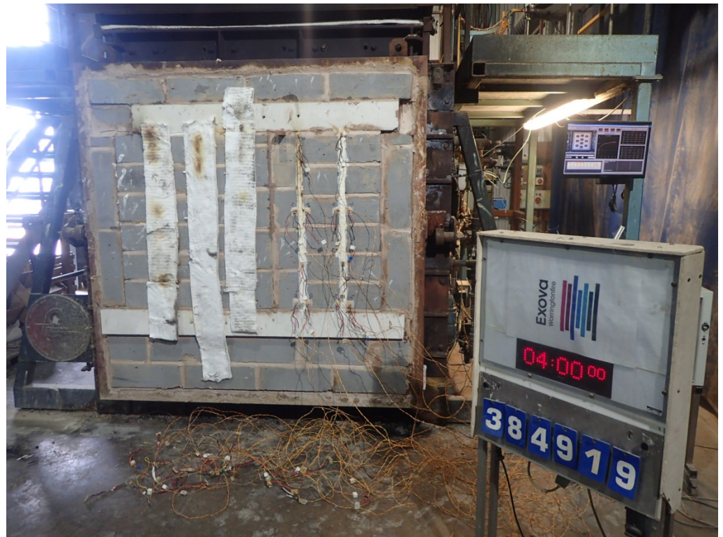
The unexposed face of the wall construction after a test duration of 240 minutes
