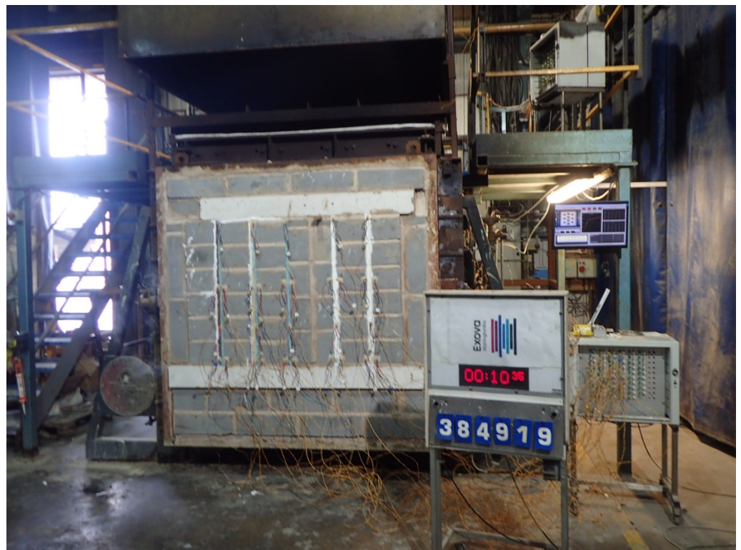
The unexposed face of the wall construction after a test duration of 10 minutes
