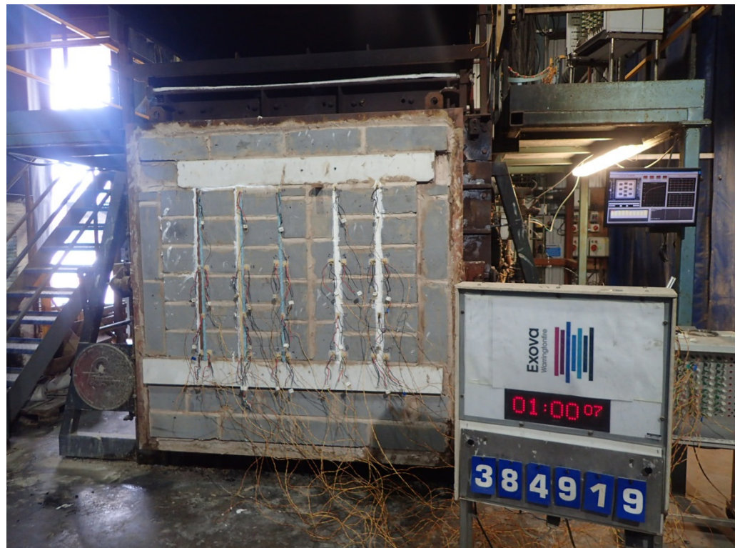
The unexposed face of the wall construction after a test duration of 60 minutes
