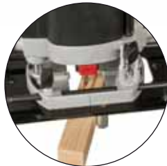
Offset mortising For timber thickness 50mm to 200mm.
