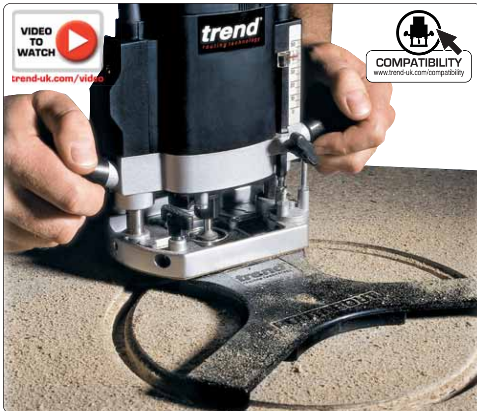
Setting-up The diameter of the finished access hole will be 250mm. Carefully mark the centre point of the circle, if possible positioning the access hatch between the floor joists. Screw the Routabout jig to the floor using a single No.8 particle board screw at the centre point to act as a pivot.
