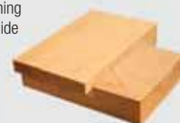
Half lap (halving) joint using tenon slide template.
