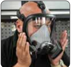
Make a face fit test by blocking the filters and inhaling to check the seal for air leakage.
