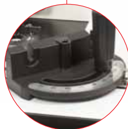
Quality Mitre Fence With zeroing and splinch block facility.
