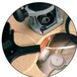
Completed cut When cut, the waste piece is supported by the wings of the jig. The stepped cutter automatically cuts a rebated edge on the waste piece as well as around the edge of the hole.
