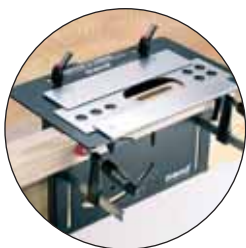
Routing the mortise
