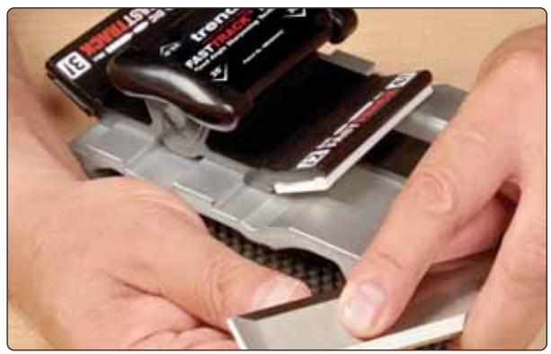
Hones square edged chisels and plane blades from 1/8" (3mm) to 2-1/2" (64mm).
