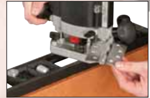
Routing hinge recesses
